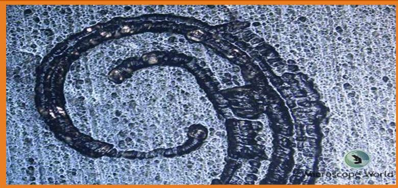
This image of a piece of metal with scratches on it was captured under a metallurgical microscope at 100x magnification.
